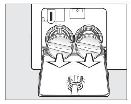
■ Remove the drain filters completely.
