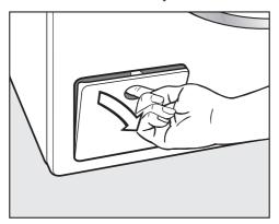
■ Open the drain pump access panel.
